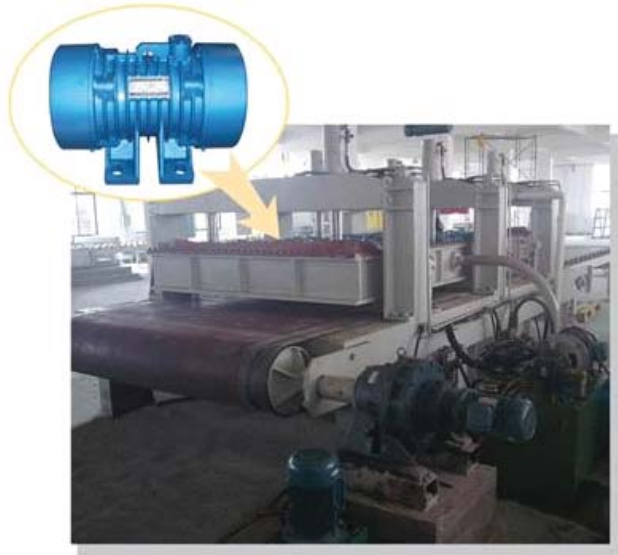
Special vibration motors in the use of artificial quartz stone presses
